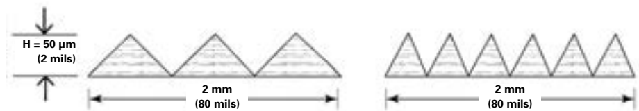
Fig. 1: Both surfaces have the same measured peak-to-valley height. A second important measurable parameter, peak density, helps explain why coatings bond differently to each surface.
