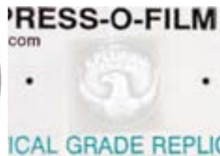
Fig. 5: Replica tape embossed over a coin (center), a digital surface image created from the tape and from a field instrument (right).
