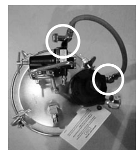
Assemble valve end of hose assembly to regulator using a 5/8 wrench. Assemble other end of hose to air motor with same wrench.
