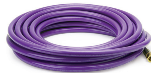
Wire-braided, 4500 psi (310 bar, 31.0 MPa) maximum working pressure rated at 180° (82.2° C)
