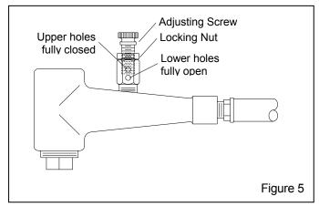
**5.3.3** If pulsation occurs in the media hose, either media is damp and caked, or not enough air is entering the media stream. While blasting, loosen the locking nut and slowly turn the adjusting screw out (counterclockwise when
