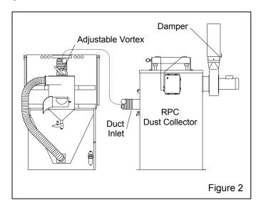
**1.5.3 Reverse Pulse Dust Collector:** A pull-through reverse-pulse dust collector is the most efficient dust collector option. Cartridge filters are automatically cleaned by a periodic pulse of compressed air. This type of dust collector used with the optional HEPA filter must be used in applications in which toxic dust is generated. See separate manual for operation of reverse-pulse dust collectors.
