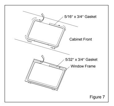
**7.4.2** Remove the window and window frame per Section 7.5.
