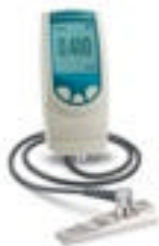
PosiTector UTG: Wall Thickness Gauge - Measures the wall thickness of materials such as steel, plastic and more using ultrasonic technology. Ideal for measuring the effects of corrosion or erosion on tanks, pipes or any structure where access is limited to one side. Multiple echo (ME) Thru-Paint models measure the metal thickness of a painted structure without having to remove the coating.
