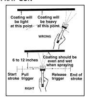
Generally use 15-20 psi air at gun inlet. Unusually heavy, difficult to atomize fluids may require up to 40 psi air at gun inlet.
