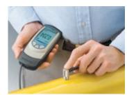
Flip Display enables right-sideup viewing whether the gage is in your hand, on your belt or on a worktable
